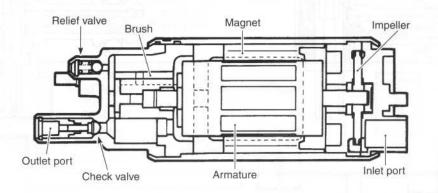
When the impeller is driven by the motor, pressure differential occurs between the front part and the rear part of the blade groove as viewed in angular direction due to fluid friction. This process continuously takes place causing fuel pressure to be built up. The pressurized fuel is then let out from the pump chamber and discharged through the motor section and the check valve.
