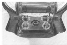
• Remove the fuel tank stay and its rubber cushion.
