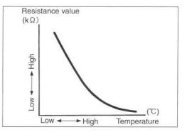
ENGINE COOLANT TEMPERATURE SENSOR (ECT SENSOR) The engine coolant temperature sensor is installed at the thermostat case.
