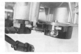
$\bullet$  Remove the idle stop screw (3).
