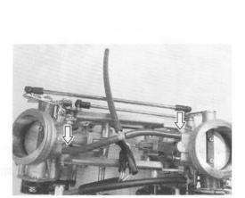
• Disconnect the STVA motor and injector couplers.
