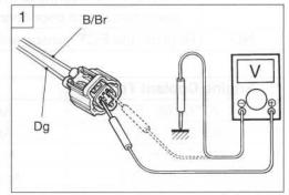
5) Measure the voltage between Dg wire terminal and ground.6) If OK, then measure the voltage between Dg wire terminal and B/Br wire terminal.
