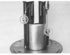
• Tighten the nuts together with the lead wire terminals.
