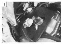
Insert the needle pointed probes to the CMP sensor coupler and crank the engine a few seconds or start the engine, and measure the peak voltage.
