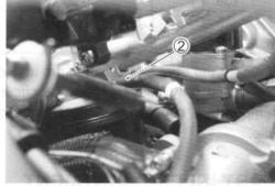
Start up the engine and keep it running at 1 200 rpm by turning throttle stop screw ③.
