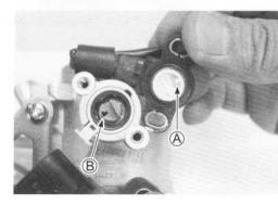
• Tighten the STP sensor mounting screws.
