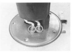
· Remove the screws and fuel level thermistor.
