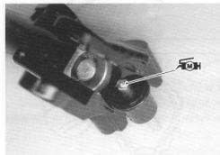
Apply SUZUKI SUPER GREASE to the bolt and pin.
