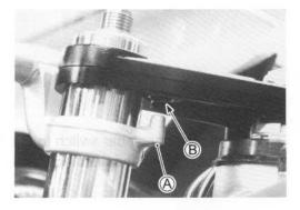
• Tighten the handlebar clamp bolts.
