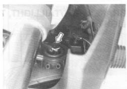
Unhook the holder spring ① and replace the headlight bulb.
